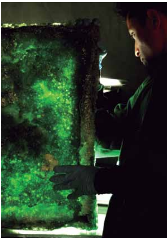
Figure 3. Large scale prototype of an ELM architectural pane
