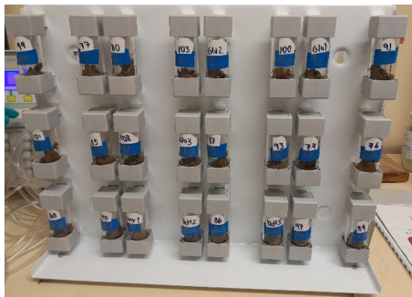
Figure 2: Setup of the respirometer system with individual capsules for each seaweed-treated soil samples ( n=48 ).
